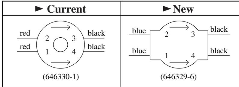
Install the Line Coil in the correct direction as illustrated below so that Lead Wires can't protrude from the space.
