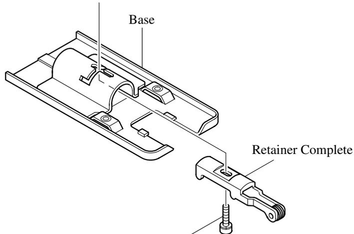
**Part No. of this Hex. Socket Head Bolt M4x16 has been changed from 266178-1 to 922128-3.**
