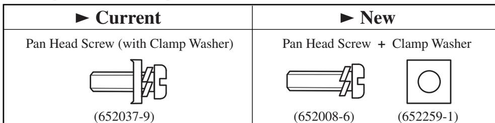
2) Clamp washer has been added to Pan head screw.
