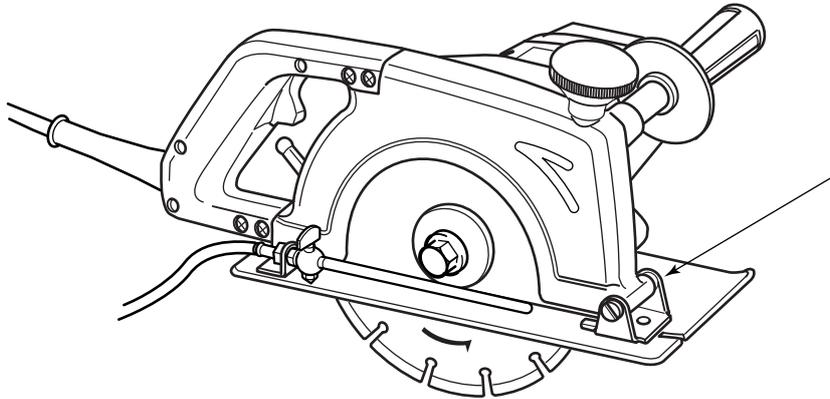
Hex. Nut, Flat Washer and Spring Washer at this hinge portion replaced by Hex. Lock Nut M6-10
