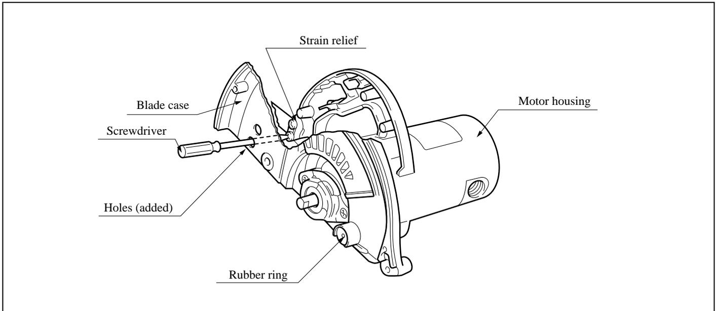
2. To increase the durability of the rubber ring which supports the safety cover (safety guard), the rubber ring 10 will be replaced by a rubber ring 8. An axis and protector (rib) for the rubber ring 8 will be added to the blade case. The pan head screw M8 (rubber ring securing screw) will be discontinued.
