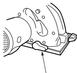
Large and easy-to-operate lever for adjusting the depth of cut
