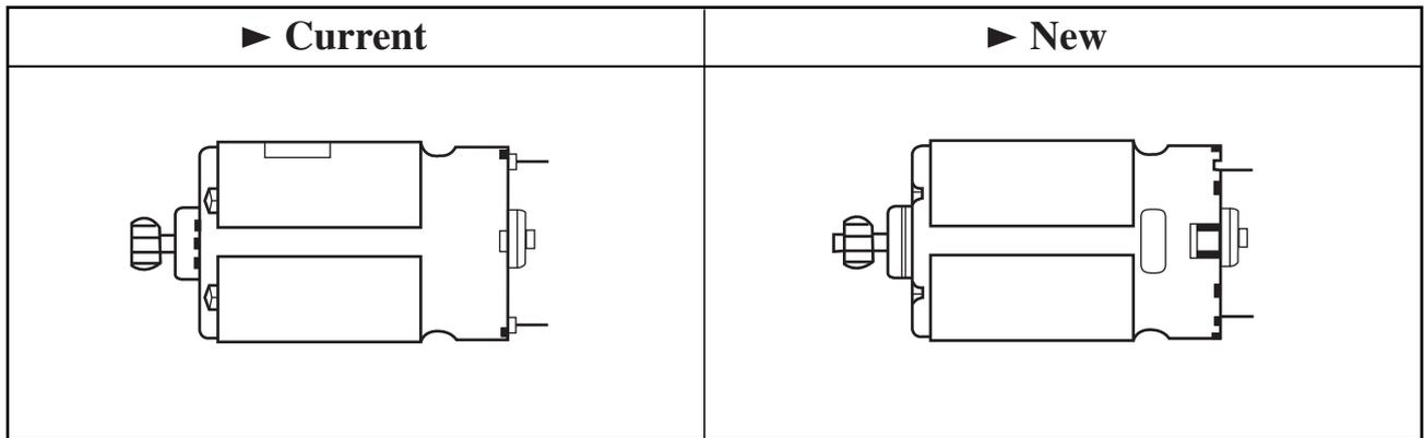
2. Position of red mark has been changed as illustrated below. Wiring and part No. of DC Motor remain unchanged.
