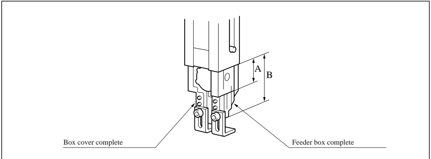
The dimensions (A) and (B) will be changed as follows so that 1-5/8" screws can be fastened.
