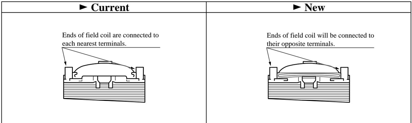
As a result, the method of connecting the lead wires to field will be changed as follows. (Note: The method of connecting the field to the switch will remain unchanged.)
