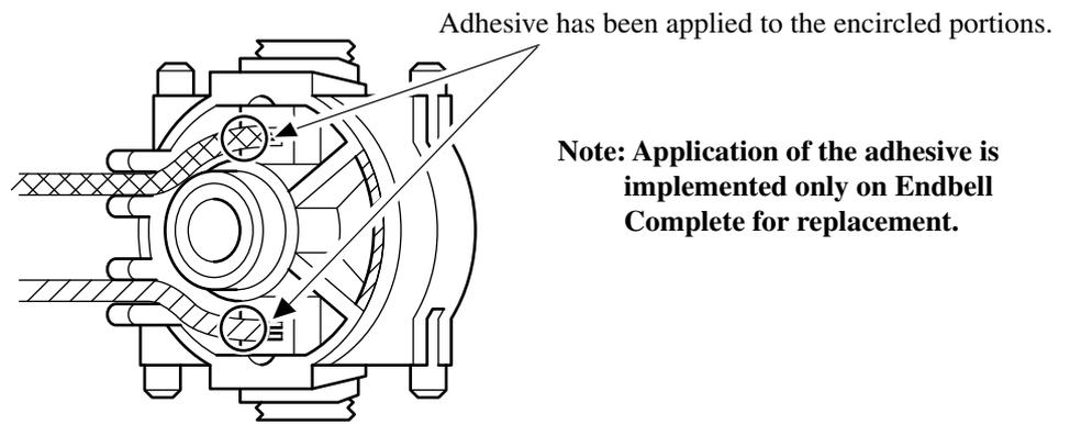
**Note: Application of the adhesive is implemented only on Endbell Complete for replacement.**
