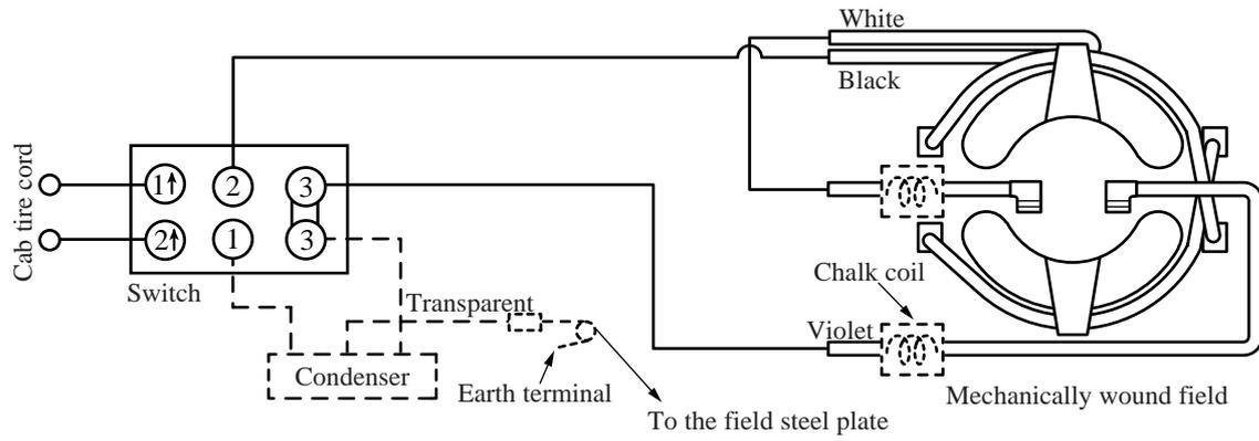
The condenser is not used in some areas and the condenser with two legs (without lead wire) is used in other areas. The chalk coil (with lead wire) is not used in some areas.
