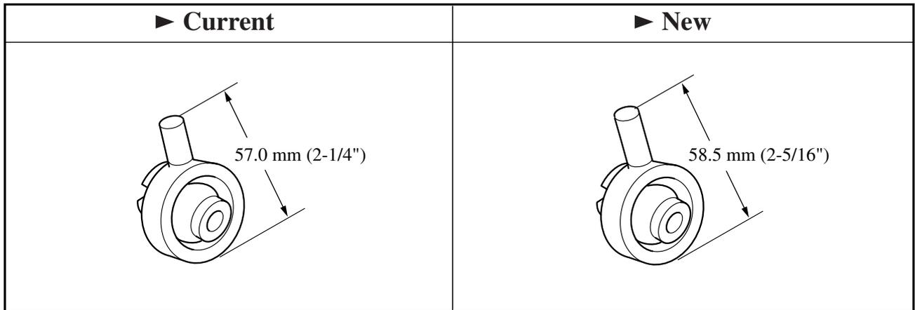
Note: New Swash Bearing 10 is available now as a replacement part. But either the current Swash Bearing 10 or the new one will be used to assemble BHR200 at our factory for a while.
