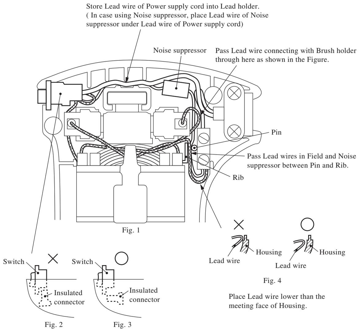
When you use Noise suppressor, place Insulated connector under Switch on its side as shown in Fig. 3 to prevent it from interference with Switch
