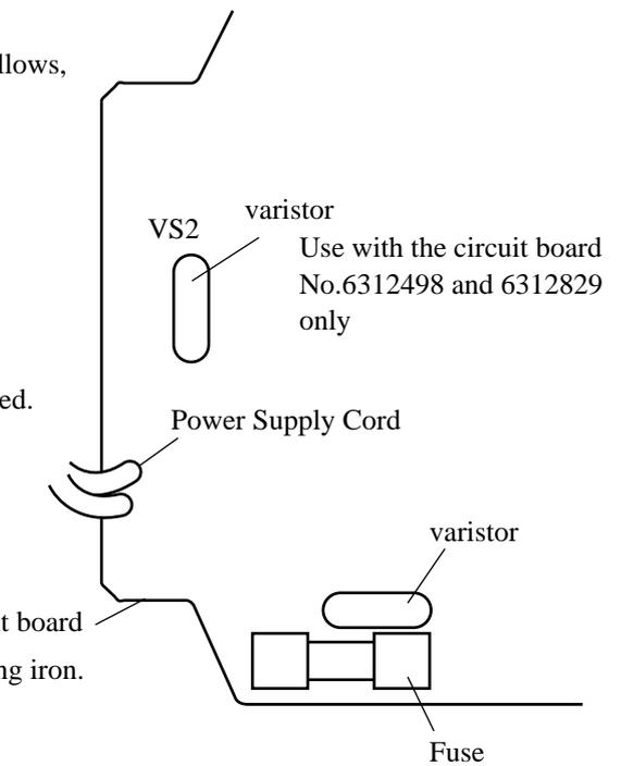
The overhang length must be under 3mm
