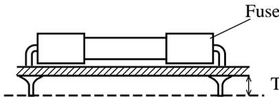
The overhang length must be under 3mm by cutting the extra.
