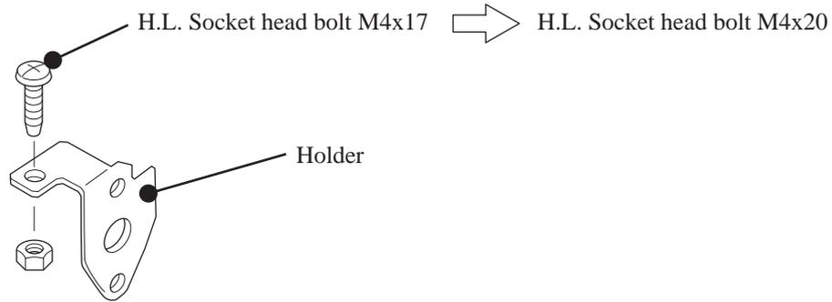
**Note:** If replacing the current part (part No. 266887-2) with a new part (part No. 266927-6), replace it together with Holder (part No. 346730-2).
