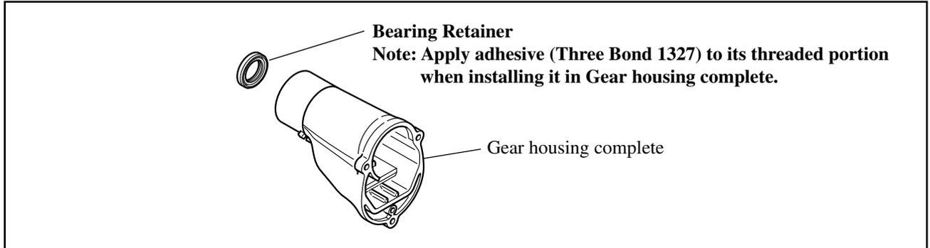
2. Shape of Gear housing cover complete has been modified as shown below.
