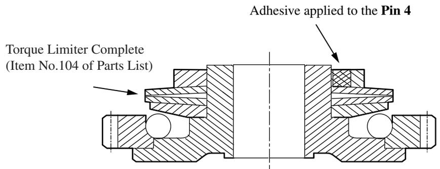
Note: Regarding Torque Limiter Complete as a replacement part please check the Torque Limiter for Pin 4's presence. When Pin 4 is not present, insert Pin 4 in the portion where the notch on the Driving Nut of the Torque Limiter meets that of a Round Nut of the Torque Limiter as shown on right. Caution: Be careful not to drop Pin 4 at the time of repairing. Please use LOC TITE 603 (Part No. 045047-7A) as a adhesive.
