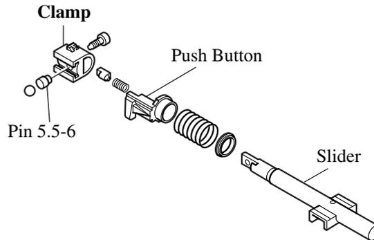
To distinguish new Clamp from current one, new Clamp has a projection as illustrated below.
