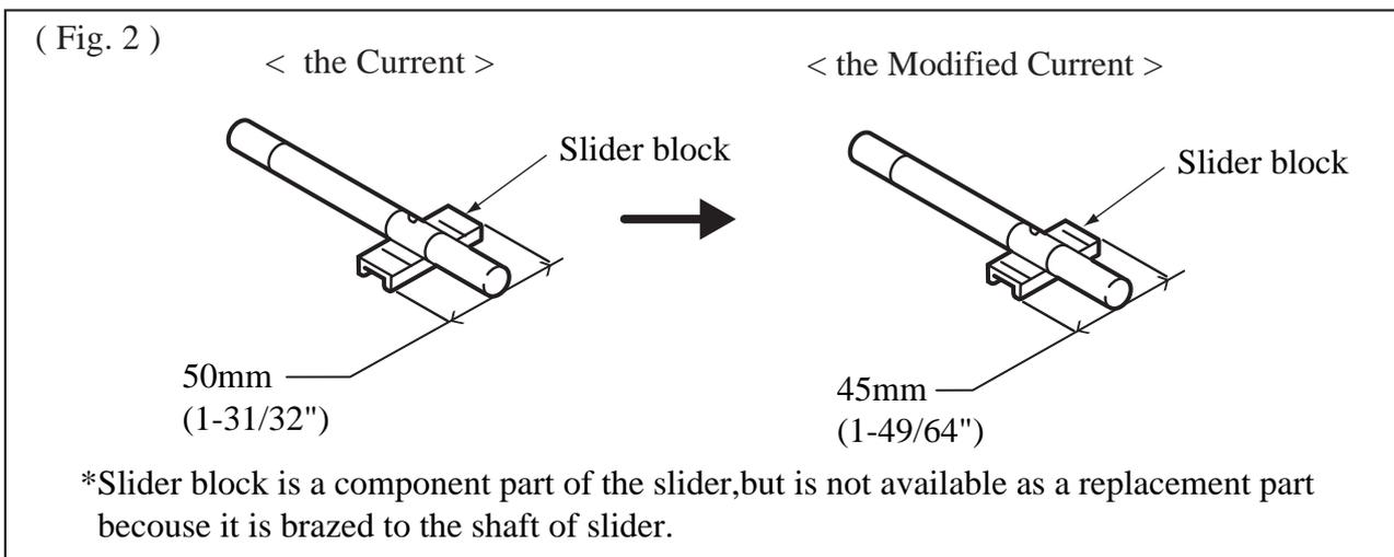
Be sure to use only the "modified current slider" for replacement of the current slider.
