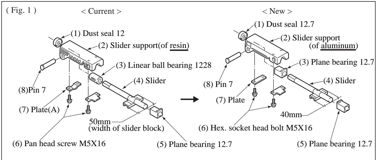
\* \*Details of Changes on Parts in Fig. 1\* \* (See List 1 about each part No. of the current/the new.)
