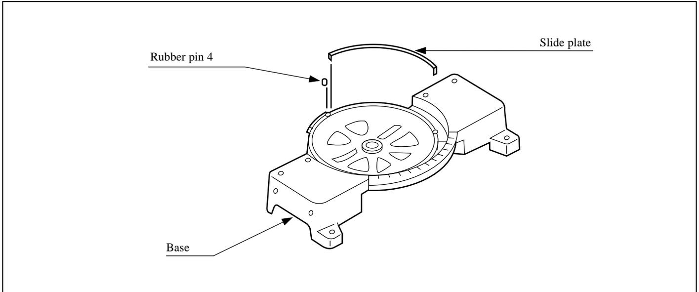
1. The slide plates will be changed from 0.3 mm (0.0012" ) to 0.5 mm (0.002" ) in thickness and 3.8 mm (5/32" ) to 6.0 mm (15/64" ) in width.
