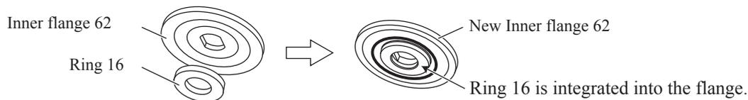
⑤, ⑥ Elimination of Ring 15.8 and Addition of Inner flange 62 from/to Standard accessories.
