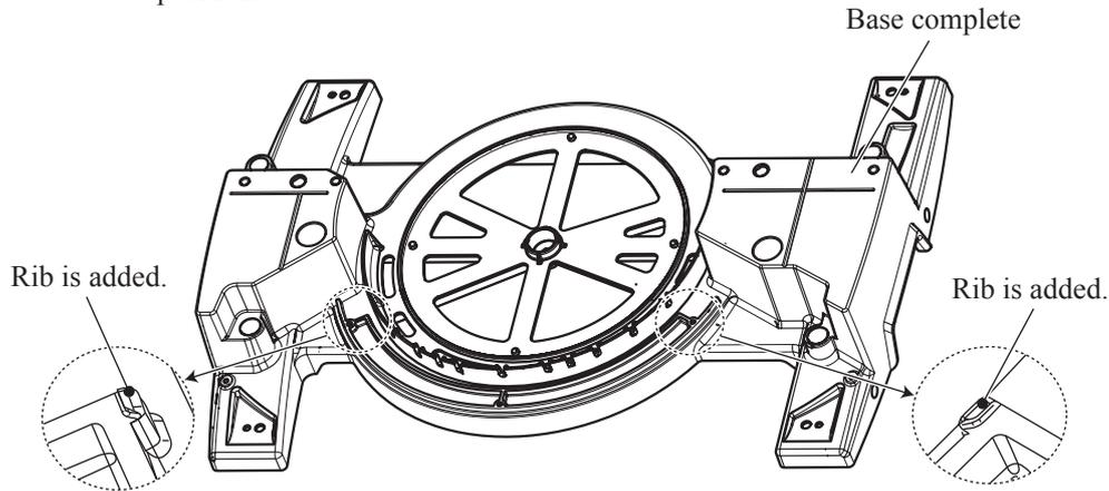
**Note in assembly:** Fasten Tapping screws while holding the edge of Miter scale plate to the ribs as follows.
