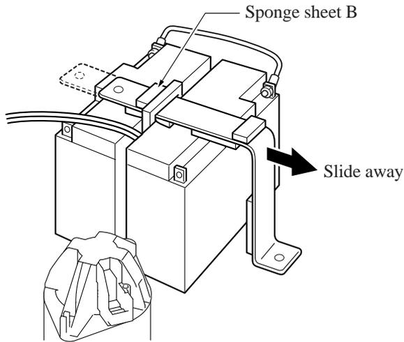
Slide the battery holder complete until the sponge sheet B touches with the temperature fuse complete.
