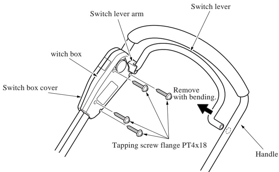
Slightly bend the switch lever and then remove the switch lever from the handle.
