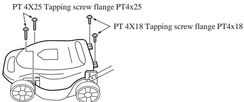
Remove the rear bag, and then loosen the tapping screw PT4x25(2 pieces) and PT4x18(2 pieces) for mounting the curling to disconnect the curling.
