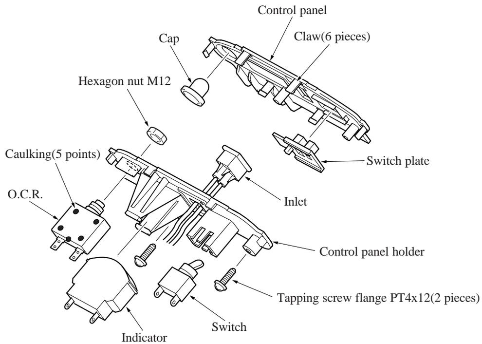
Loosen the tapping screw flange PT4x12(2 pieces) to remove the claws at 6 points, and then disassemble the control panel and control panel holder.
