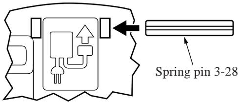
Insert the spring pin 3-28 in the direction shown on the figure and then mount the inlet cover.
