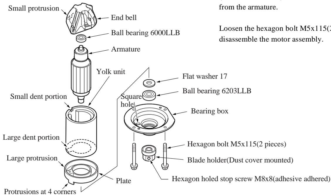
Loosen the hexagon holed stop screw M8 x 8 (Adhesive attached) to remove the blade holder from the armature.
