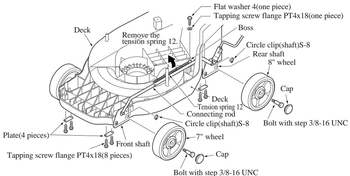
Remove the wheel cap and then loosen the bolt with step 3/8-16 UNC to disconnect the 7" wheel and 8" wheel. Loosen the tapping screw flange PT4x12(1 piece) to remove the flat washer 4. Remove the tension spring 12 from the boss on the deck. Remove the circle clip(shaft)S-8 from the front and rear shafts. Remove the connecting rod.
