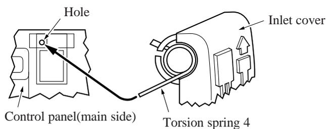
Set the torsion spring 4 on the inlet cover as shown on the figure and then insert the longer arm of the torsion spring 4 through the hole of control panel.
