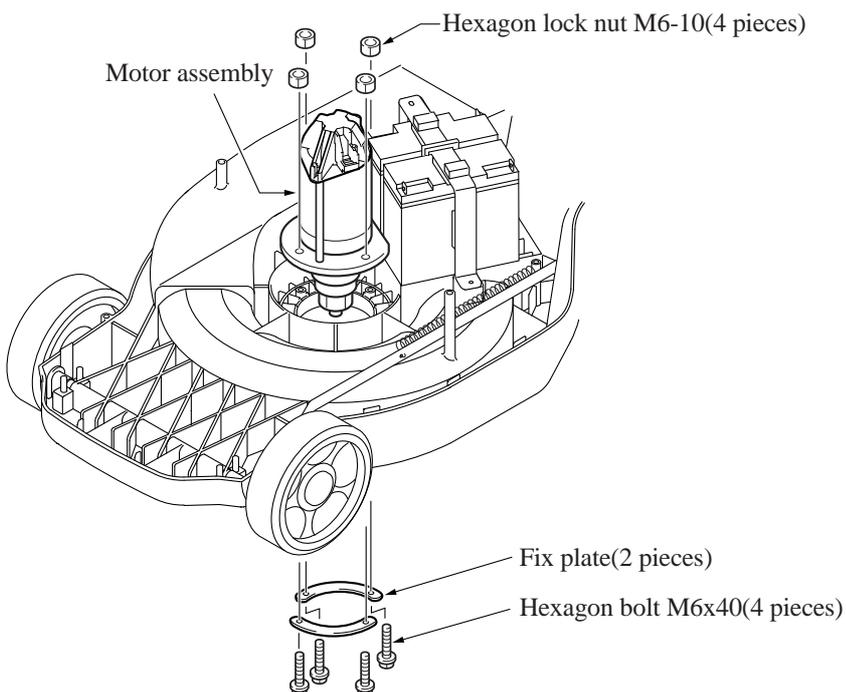
Engage the box wrench 10 with both hexagon lock nut M6-10 and hexagon bolt M6x40, and then disassemble the hexagon bolt M6x40 and the fix plate.
