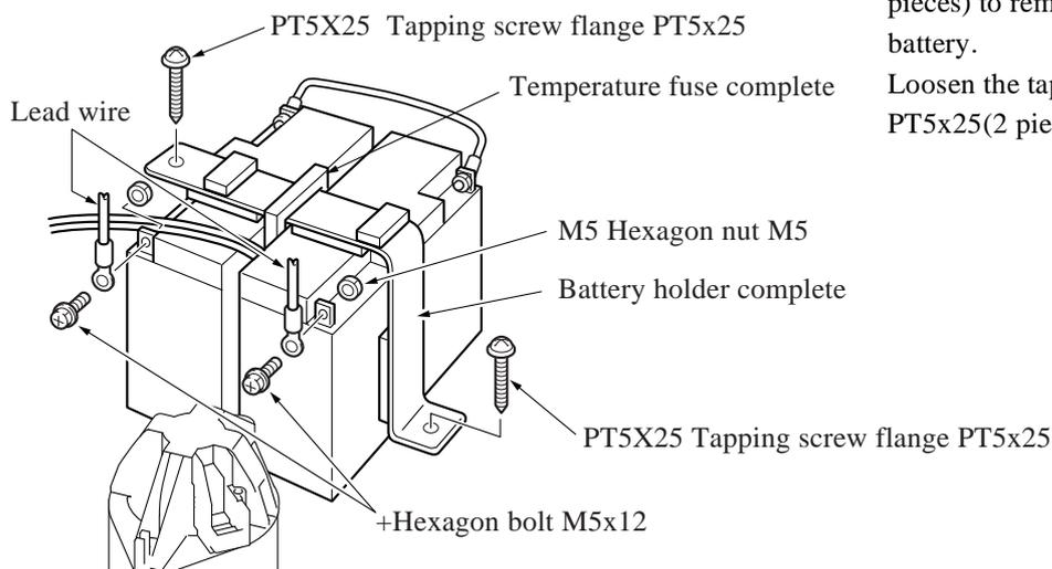
Loosen the +Hexagon bolt M5x12(2 pieces) to remove the lead wire from the battery.
